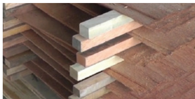
Coconut Veneer laid up prior to drying. Source : 7
