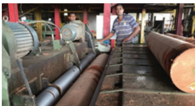
Debarked and rounded coconut logs set in spindleless lathe ready for peeling into veneer. Source: 6
