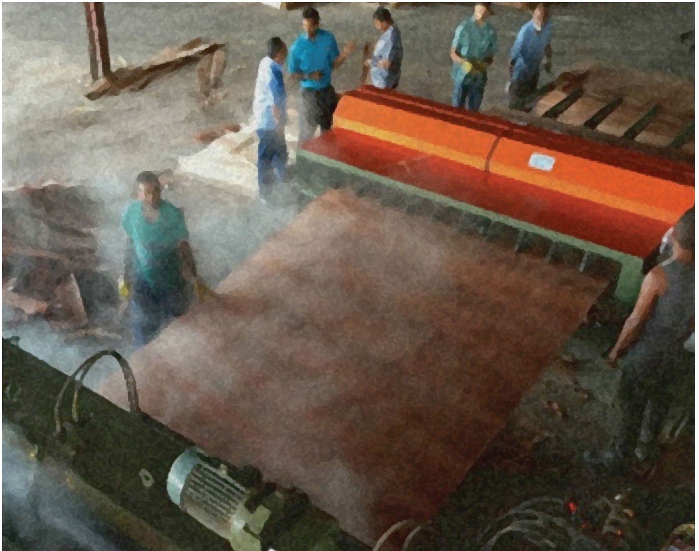
Green veneer sheet fed from spindleless lathe and prior to clipping. Source: 10
