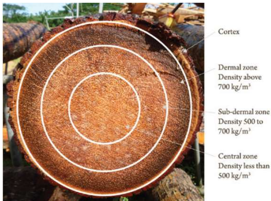
Figure 1: Cross-section of coconut palm showing vascular bundling (density distribution) from centre to the outer cortex. Adopted from McGavin et al. [19].
