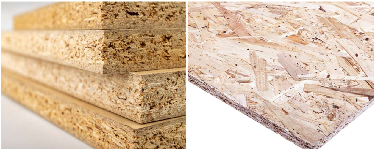
Figure 8: Particle-based product examples (Left – particleboard, Right – OSB).
