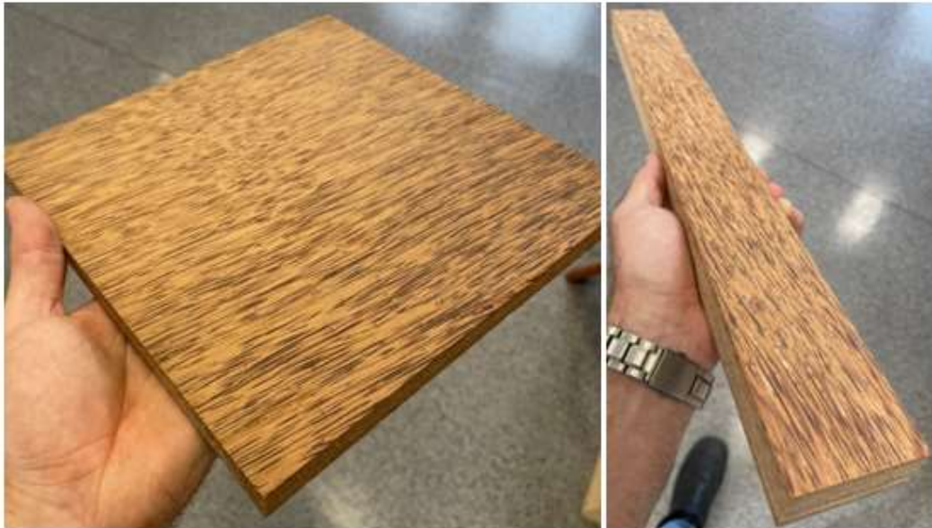
Figure 10: Structural cocoveneer EWPs: plywood (left) and LVL (right) products.
