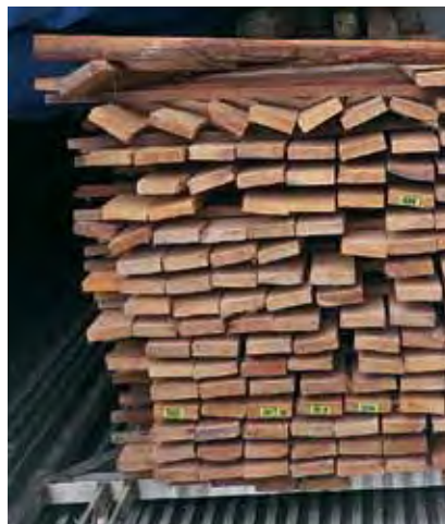
Twisted boards in an un-weighted stack
