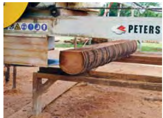
Board 2 removed, ready to turn
