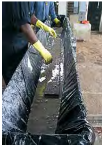
Dipping a board in a fungicide solution
