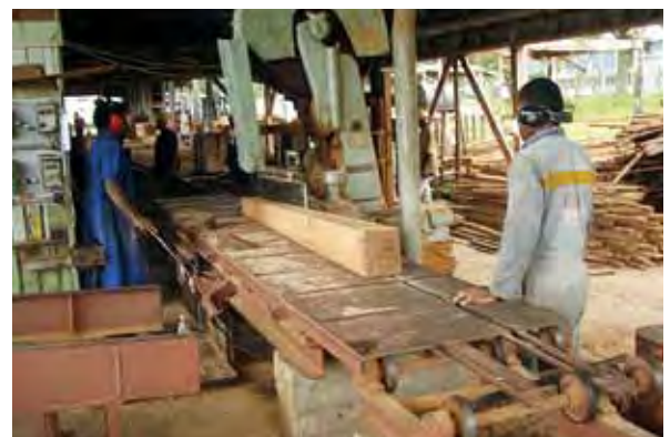
Fixed band-saw; high density boards removed
