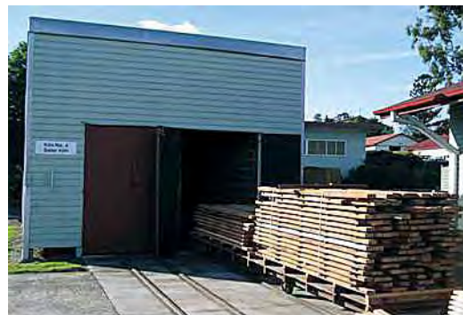
Stack ready for drying in a solar kiln. Weights still to be added.
