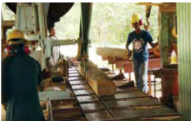
Fixed band-saw; cut 3 completed
