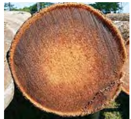
A dark band of high density wood
