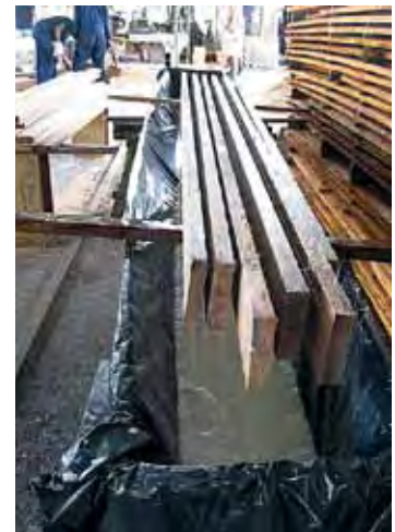
Draining boards before stacking
