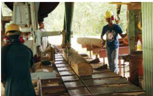
Fixed band-saw; cut 3 completed
