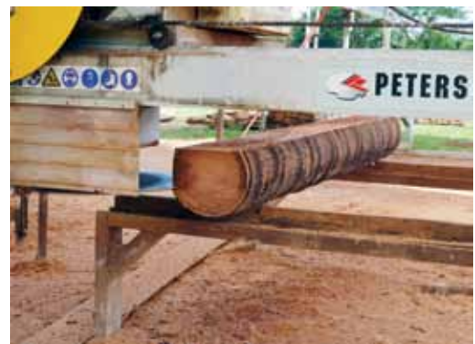
Board 2 removed, ready to turn
