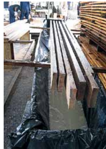
Draining boards before stacking
