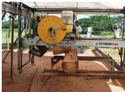
Cut 2 to produce board 1
