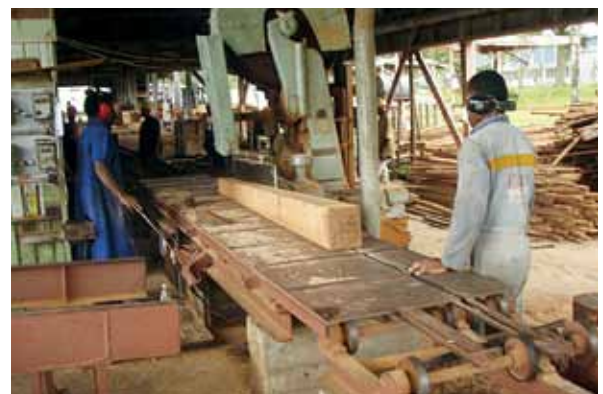
Fixed band-saw; high density boards removed
