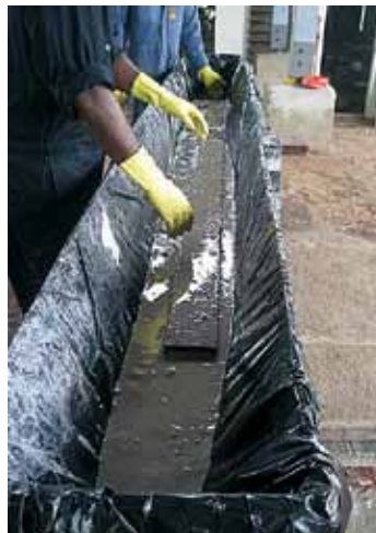
Dipping a board in a fungicide solution
