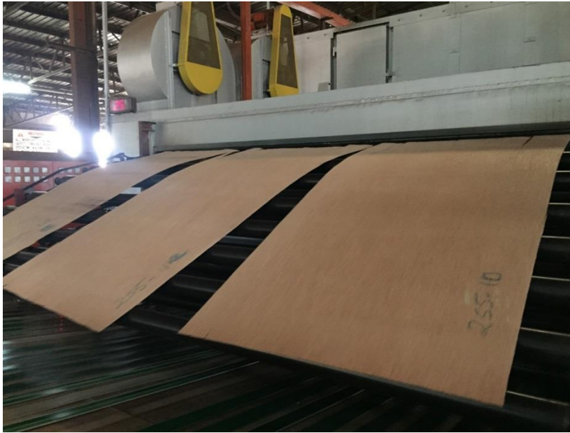
Image 3. Rotary-peeled cocoveneer exiting the jet box drier
