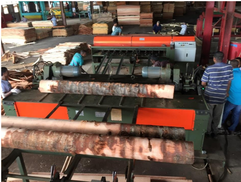
Image 1. Veneer processing using a spindleless rotary veneer lathe
