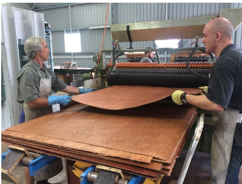
Image 7. Adhesive being applied to cocoveneer
