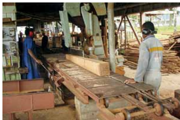
Fixed band-saw; high density boards removed
