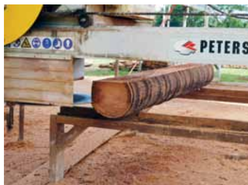
Board 2 removed, ready to turn
