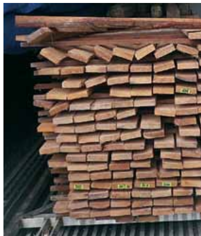
Twisted boards in an un-weighted stack
