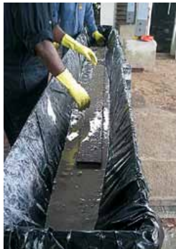
Dipping a board in a fungicide solution
