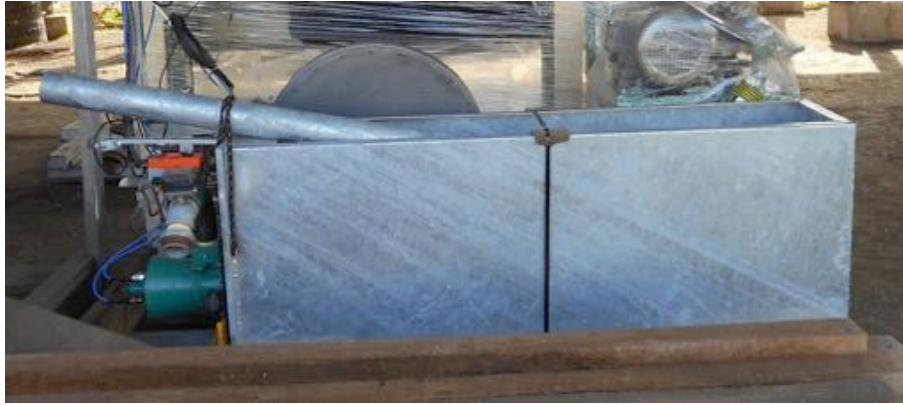
Figure 13: Steam generation unit
