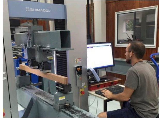
Figure 7: Coconut laminated veneer lumber (LVL) being tested for stiffness and strength.
