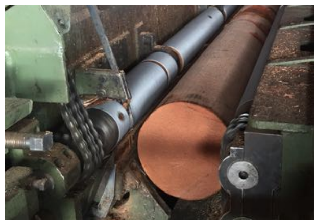
Figure 5: Harvested coconut stems being peeled using a spindle-less lathe
