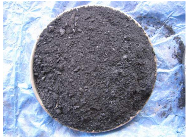
Figure 3: Crushing biochar in a modified food grinder and the crushed cocowood biochar.
