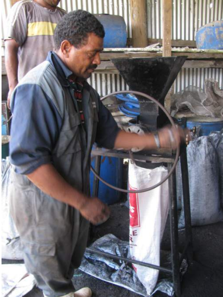
Figure 3: Crushing biochar in a modified food grinder and the crushed cocowood biochar.
