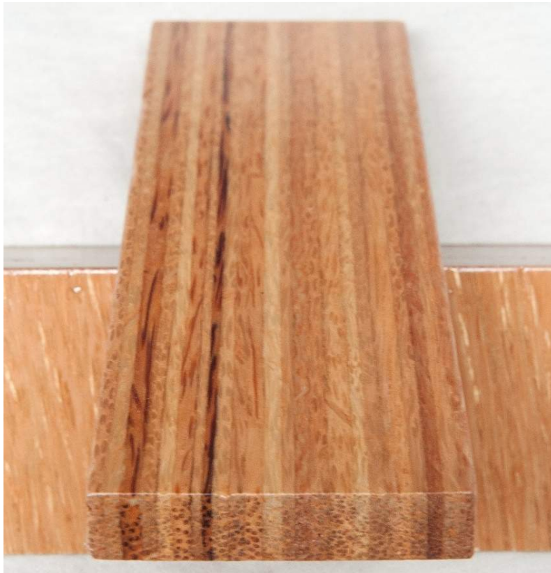
Image 13. Multilaminar wood section sawn longitudinally at 90 degrees to the veneer direction.
