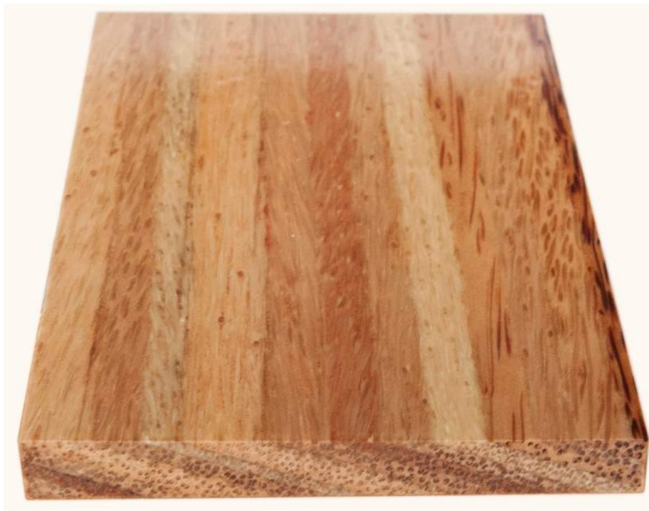
Image 14. Multilaminar wood section sawn longitudinally at 20 degrees to the veneer direction.
