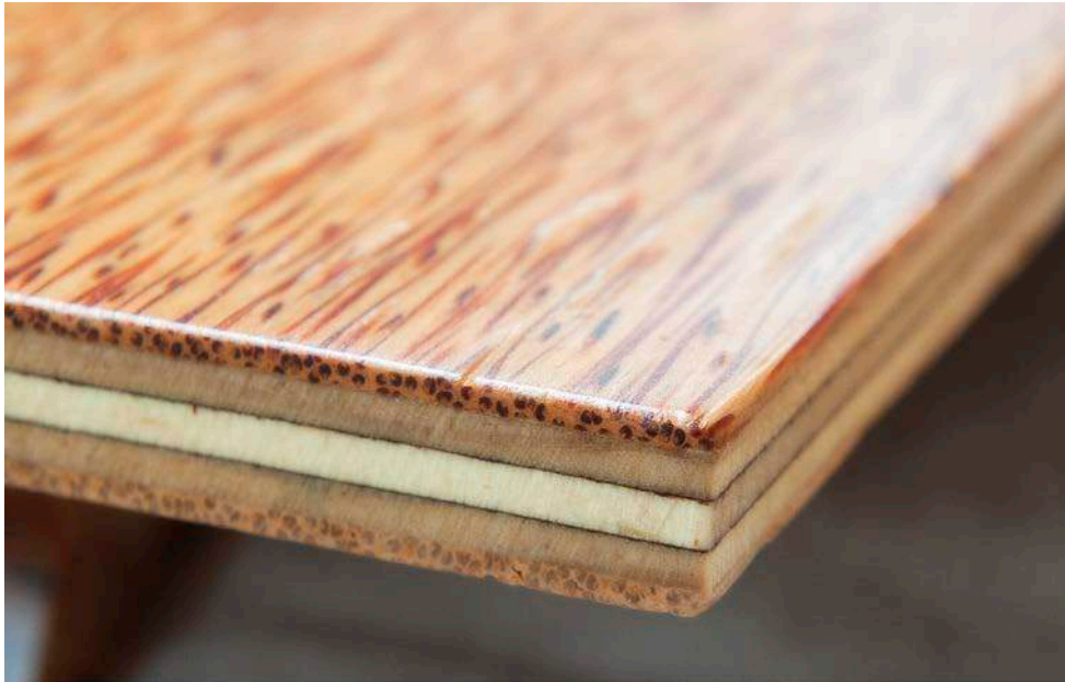
Image 3. Cocoveneer blended with other forest resources in a plywood construction.
