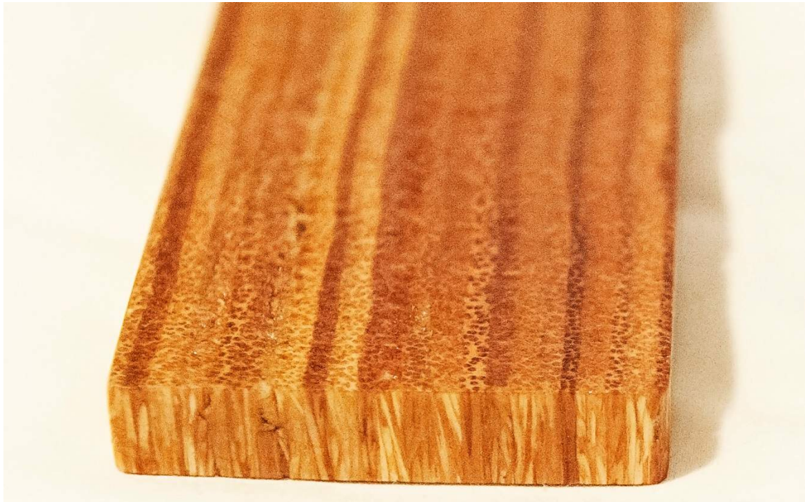
Image 15. Multilaminar wood section sawn across the grain at 90 degrees to the veneer direction.
