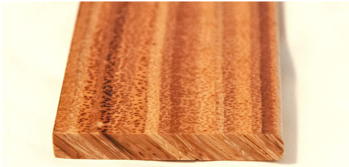
Image 16. Multilaminar wood section sawn across the grain at 45 degrees to the veneer direction.
