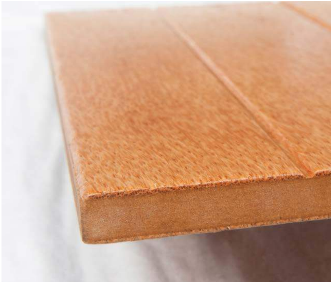
Image 5. Veneer overlay panel using medium density cocoveneer on MDF.
