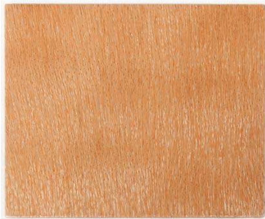
Image 6. Flat overlay panel using medium density cocoveneer on MDF.
