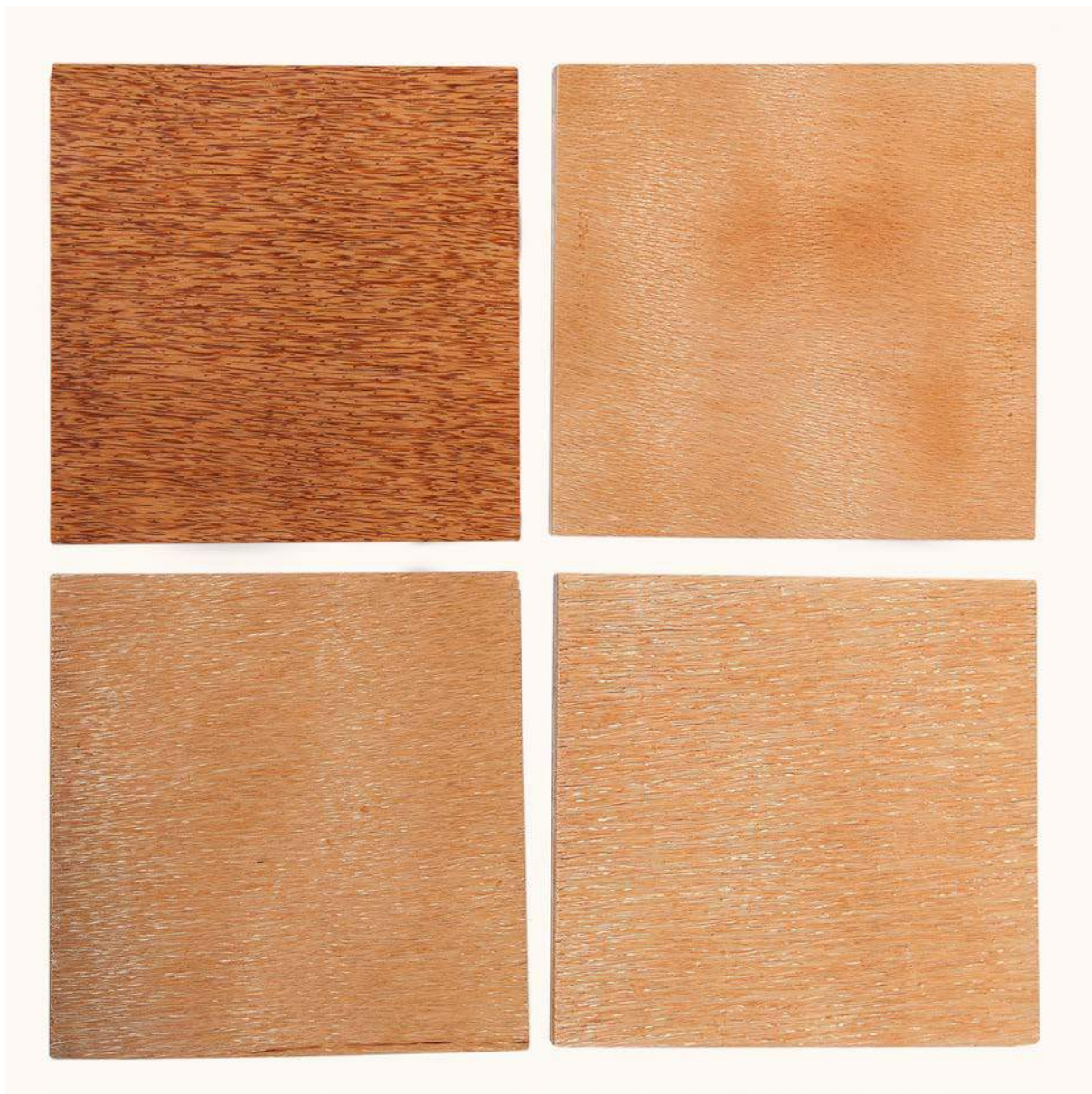
Image 2. Example of high density (top left), medium-high density (top right), medium density (bottom left) and low density (bottom right) cocoveneer face veneer in a plywood construction.
