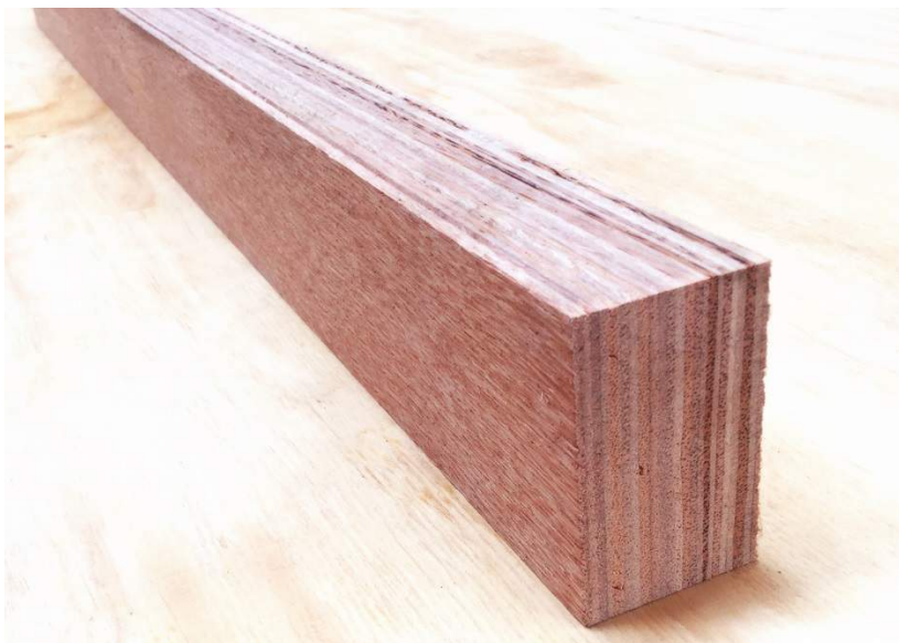
Image 4. Laminated veneer lumber manufactured from cocoveneer.
