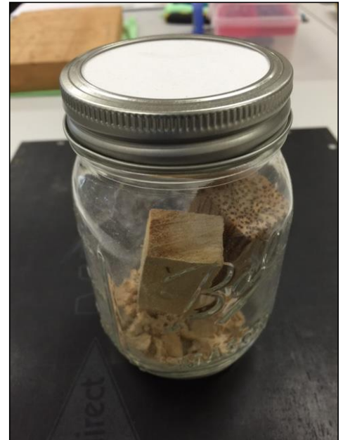
Image 7. L. brunneus adults on a control test block before being placed in a glass jar with a cocowood test block and some culture medium.
