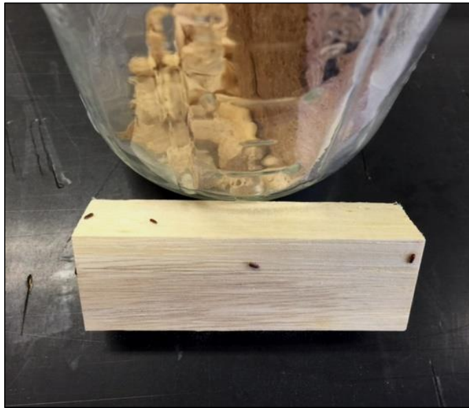
Image 7. L. brunneus adults on a control test block before being placed in a glass jar with a cocowood test block and some culture medium.
