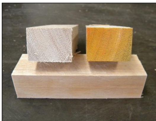
Image 2. Sapwood blocks of spotted gum with the block on the right sprayed with methyl orange to confirm a high percentage of sapwood. Yellow colour confirms sapwood.
