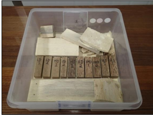
Image 8. Cocowood and blackbean control blocks were placed in plastic storage containers with sections of lyctid-infested blackbean sapwood.
