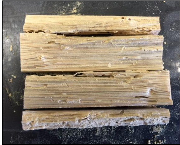
Image 17. Live lyctid beetle found emerging from a spotted gum control block – subsequent destructive sampling revealed a larval gallery and powdery frass.
