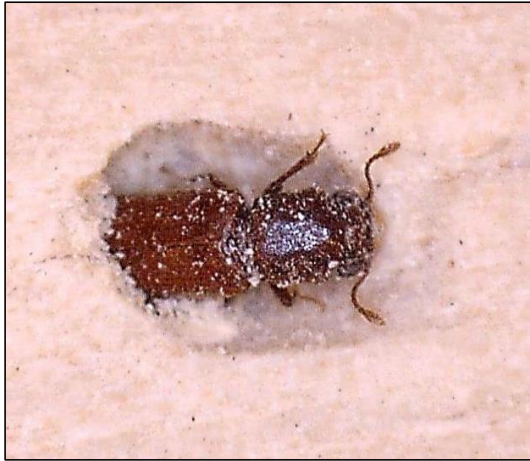
Image 17. Live lyctid beetle found emerging from a spotted gum control block – subsequent destructive sampling revealed a larval gallery and powdery frass.
