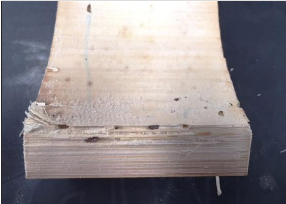
Image 26. Fresh larval galleries and live adults confirming active infestation in bamboo rings at the completion of the exposure period.
