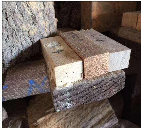
Image 18. Blackbean control block with lyctid beetle infestation externally visible adjacent to a cocowood block.
