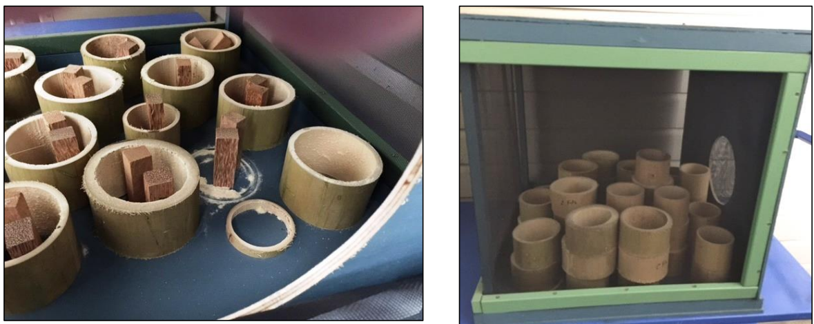
Image 15. Bamboo rings with active borer infestation (note the build-up of powdery frass) were used in a cage trial with cocowood blocks of varying densities.
