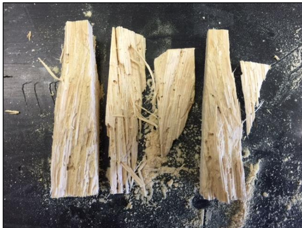
Image 20. Destructive sampling of a blackbean control block uncovered larval galleries packed with fine powdery frass.
