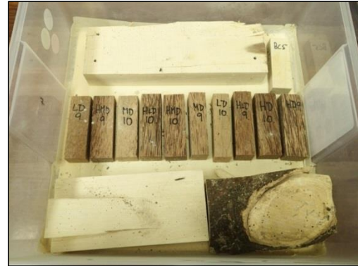
Image 8. Cocowood and blackbean control blocks were placed in plastic storage containers with sections of lyctid-infested blackbean sapwood.
