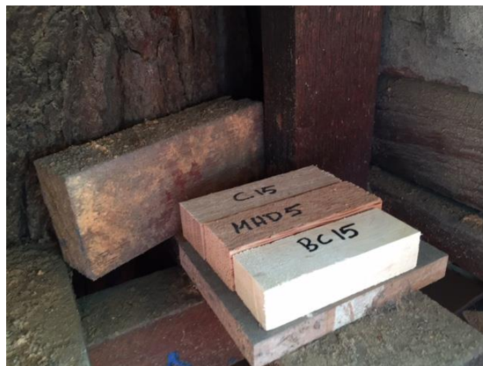
Image 3. A cocowood test block adjacent to a spotted gum (C) and blackbean (BC) control block in a timber storage area at the DAF Salisbury Research Facility.
