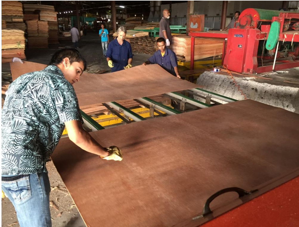
Image 3 – Veneer sheets were labelled with an individual identifier immediately after clipping
