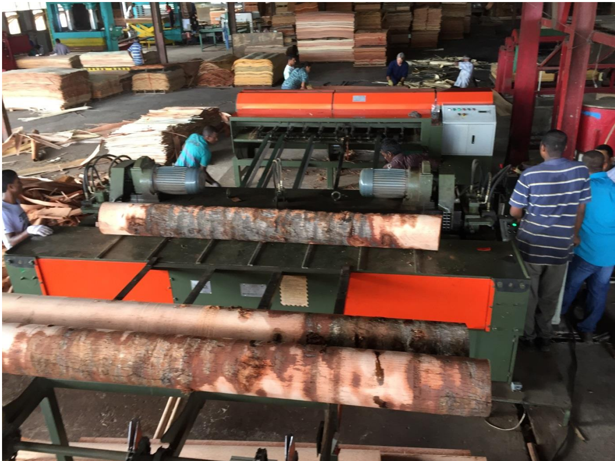
Image 2 – Spindleless veneer lathe used for peeling coconut stems
