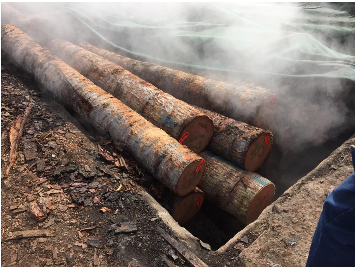
Image 1 – Water-steam chamber used to pre-condition coconut palm stem logs prior to peeling
