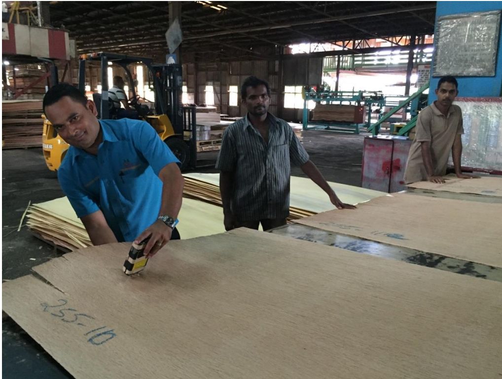
Image 5 – Checking cocoveneer moisture content at the completion of drying.
