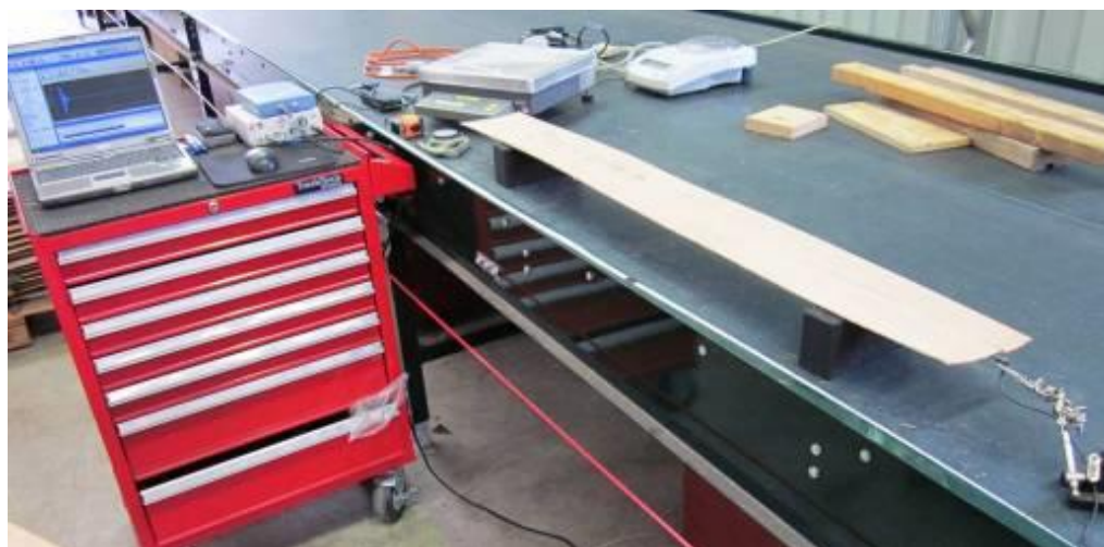
Image 6 – Modulus of elasticity measurement on cocoveneer sampling strips.
