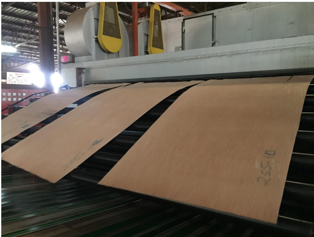
Image 4 – Cocoveneer sheets exiting the jet box drier
