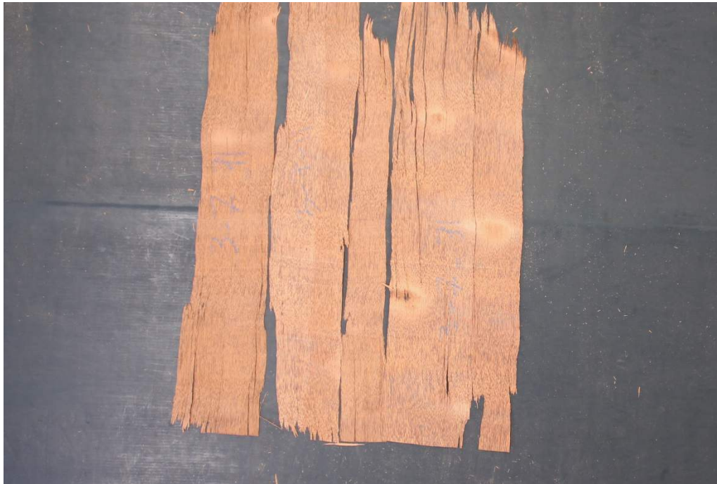
Image 9 – Example of poor quality and split veneer due to brittleness
