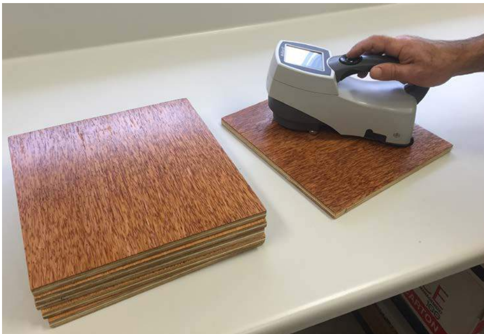
Image 7 – Colour measurement on cocoveneer
