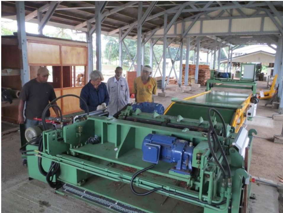
Image 15 – Introductory training provided in veneer lathe setup
