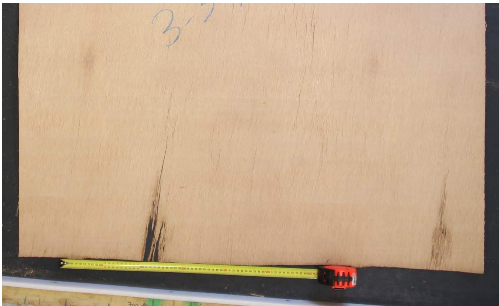
Image 11 – Example of decay in veneer
