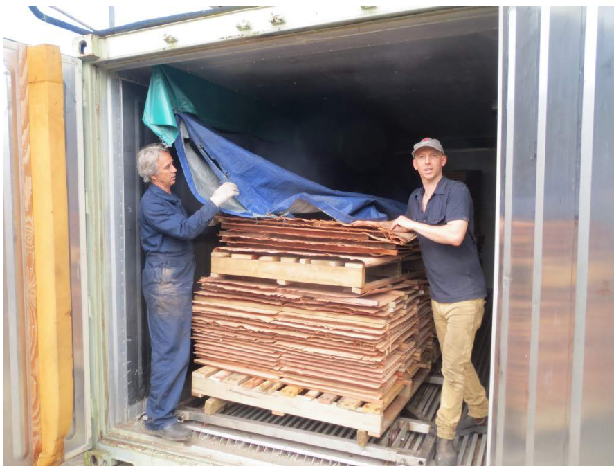
Image 4 – Cocoveneer was dried using conventional solid wood drying protocols.
