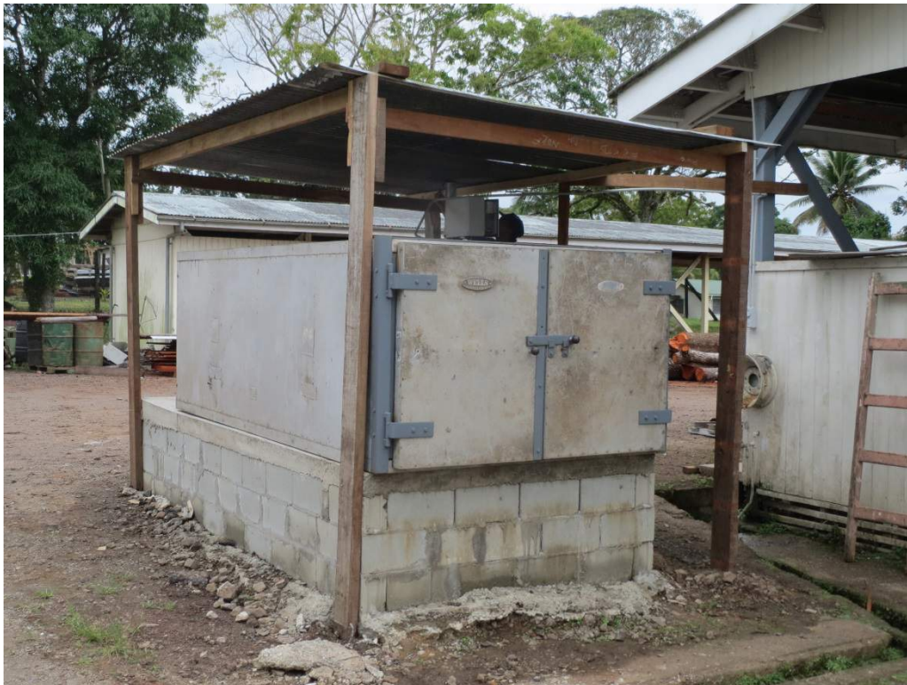
Image 1 – Chamber used to pre-condition coconut palm stem logs prior to peeling
