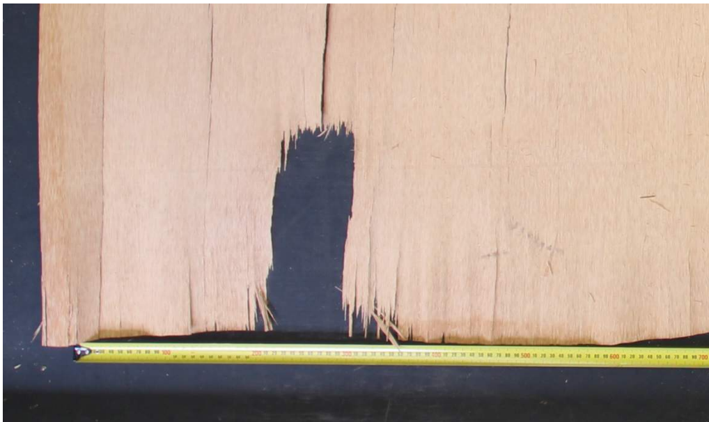
Image 12 – Example of tear-out in veneer
