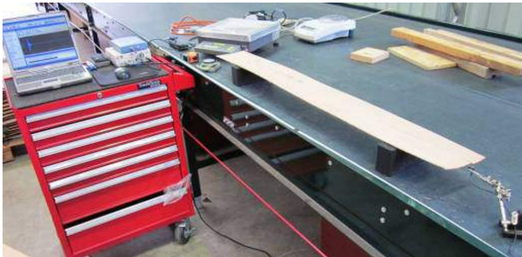
Image 5 – Modulus of elasticity measurement on cocovenier sampling strips.
