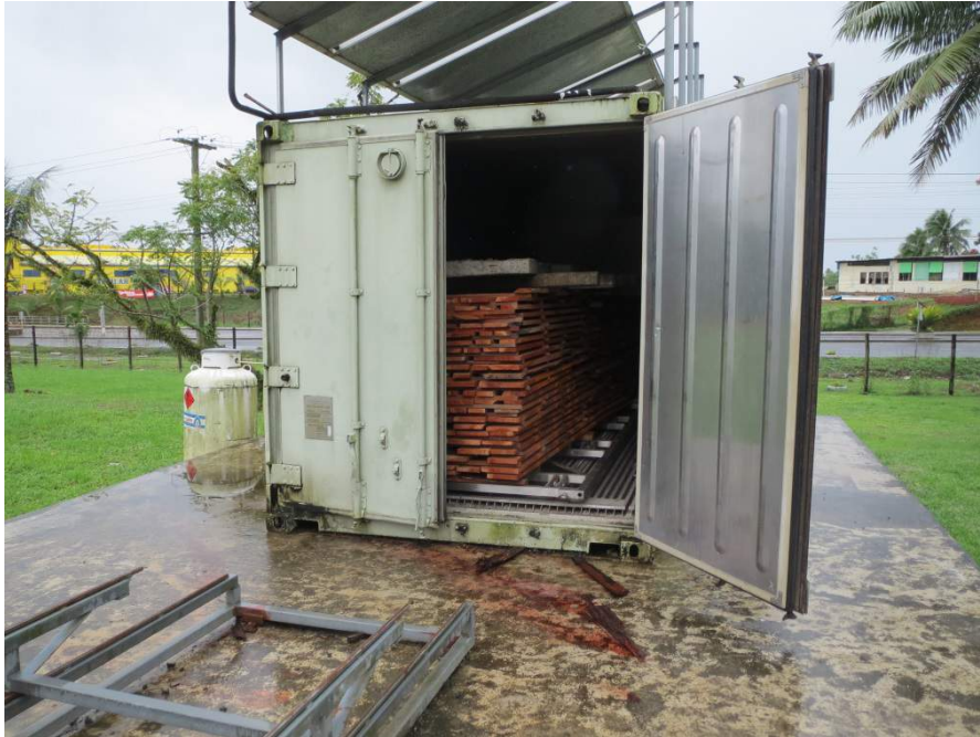
Image 3 – Gas-assisted solar kiln designed for solid timber drying.
