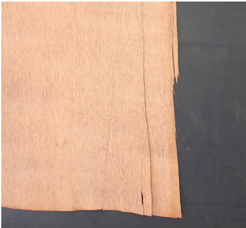
Image 13 – Example of handling splits
