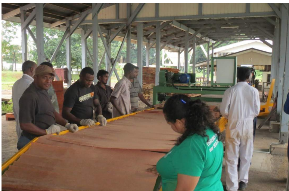
Image 6 – Cocoveneer produced on a spindleless veneer lathe
