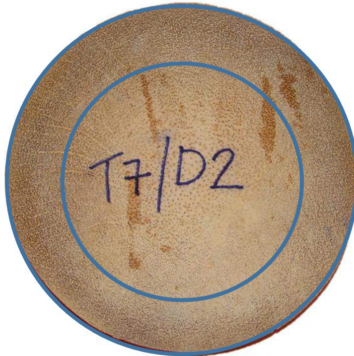
Fig. 1. Coconut disc with its specimen reference showing that the most valuable area for high density veneer production lies between the blue circles
