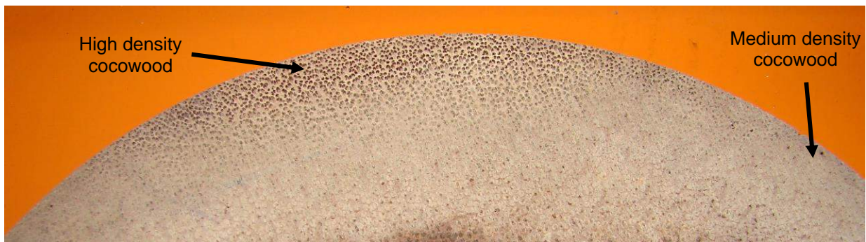
Fig. 13. Circumferential cocowood density variation
