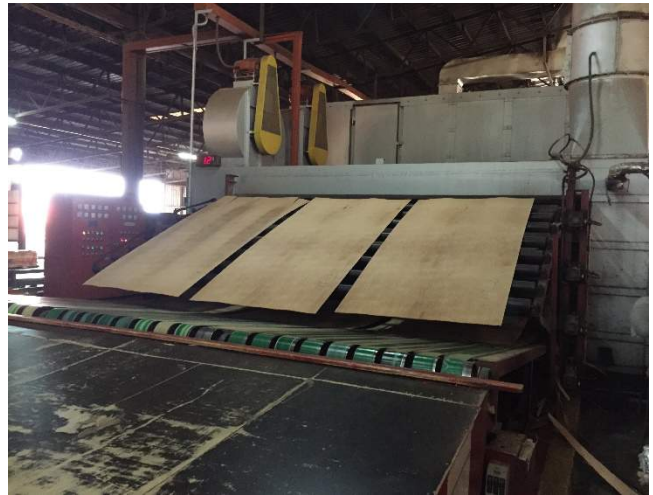
Figure 6.5 Cocoveneer dried using a jet-box veneer dryer.
