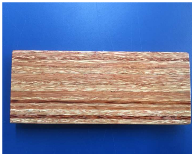
Figure 2.9 Sawn section from cocoveneer multilaminar block.
