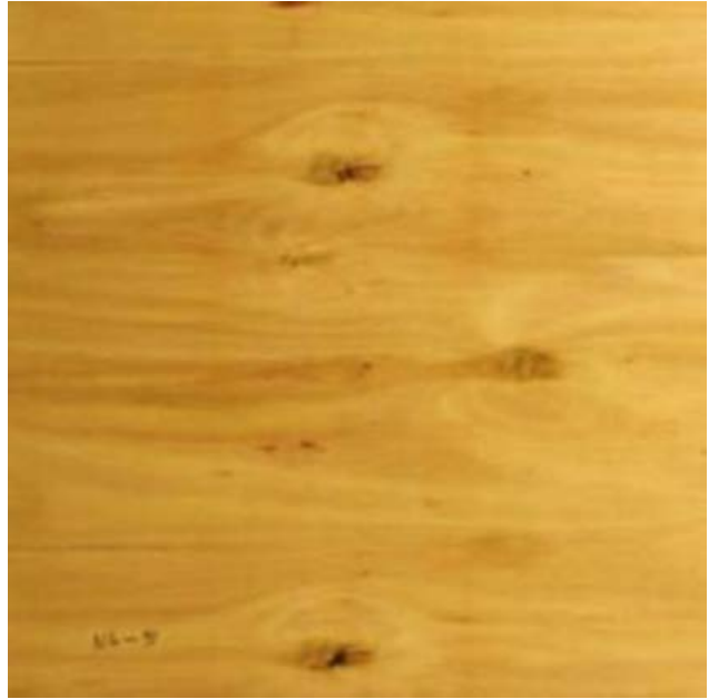
Figure 7.9 Example of the visual quality of C-grade hardwood veneer.
