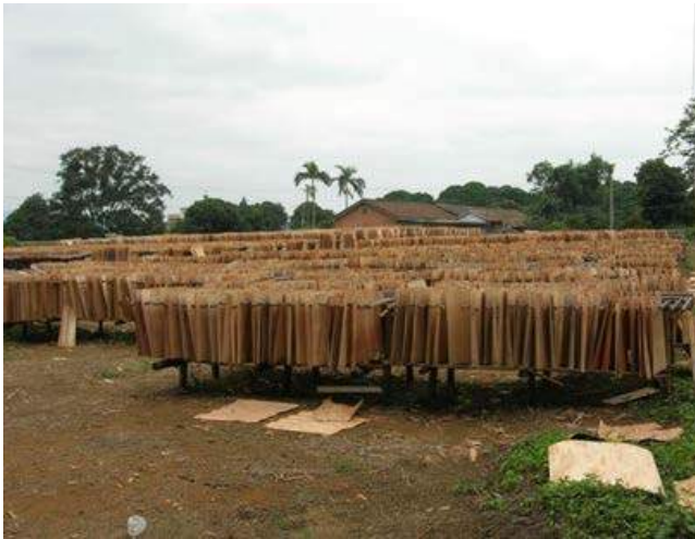
Figure 6.4 Air drying veneer sheets in Vietnam.
