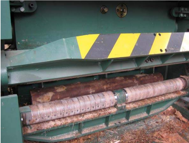
Figure 5.4 An example of a spindleless lathe.
