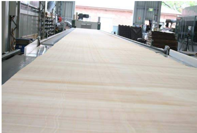
Figure 6.3 Veneer ribbon ready for clipping.
