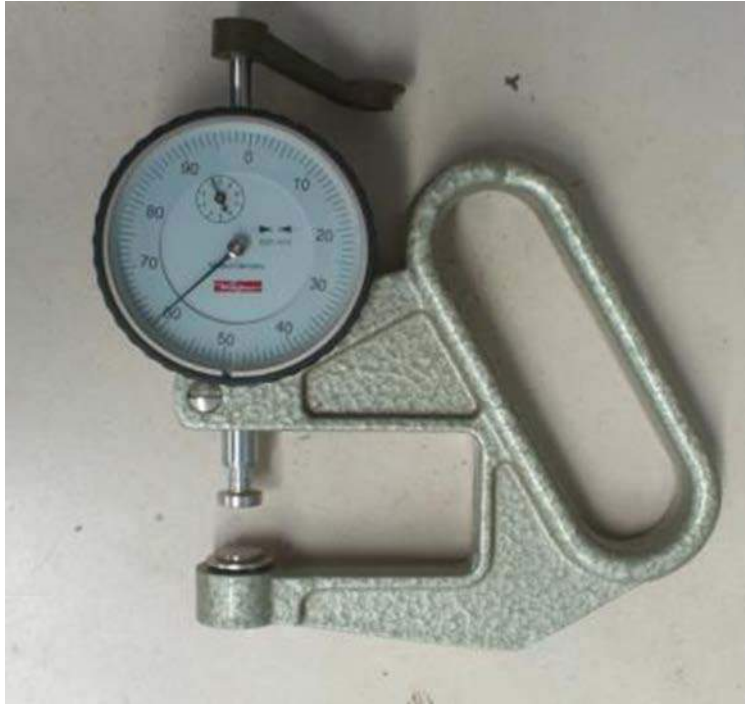
Figure 8.4 A Kafer hand-held dial gauge thickness checker.
