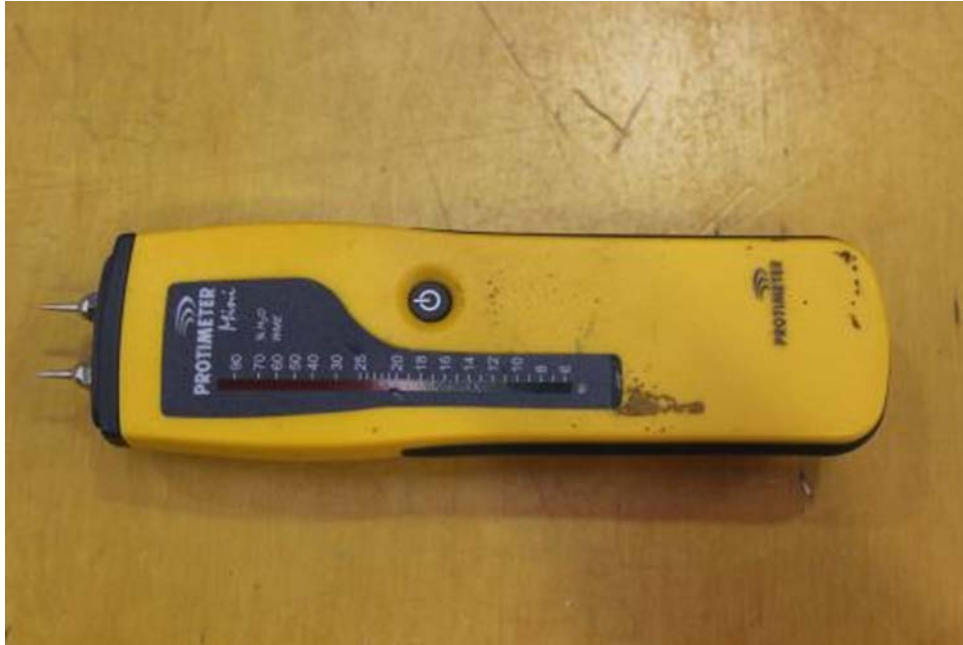
Figure 8.7 A hand-held resistance moisture meter.
