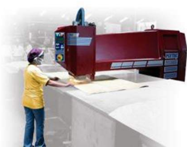
Figure 7.14 Semi- (left) and fully-automated veneer patching.
