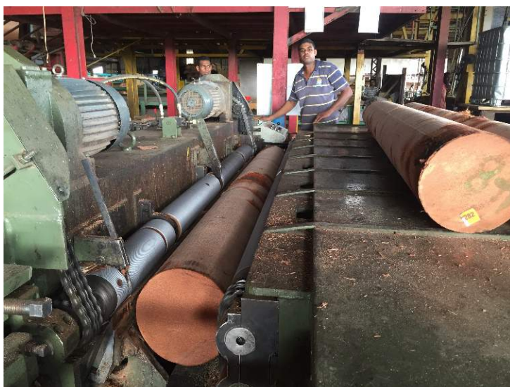
Figure 5.6 Coconut log being peeled with a spindleless lathe.
