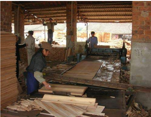
Figure 6.1 Veneer sheets being clipped manually with guillotine in Vietnam.
