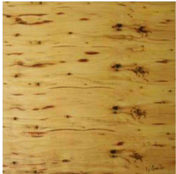
Figure 7.11 Example of the visual quality of F-grade hardwood veneer.
