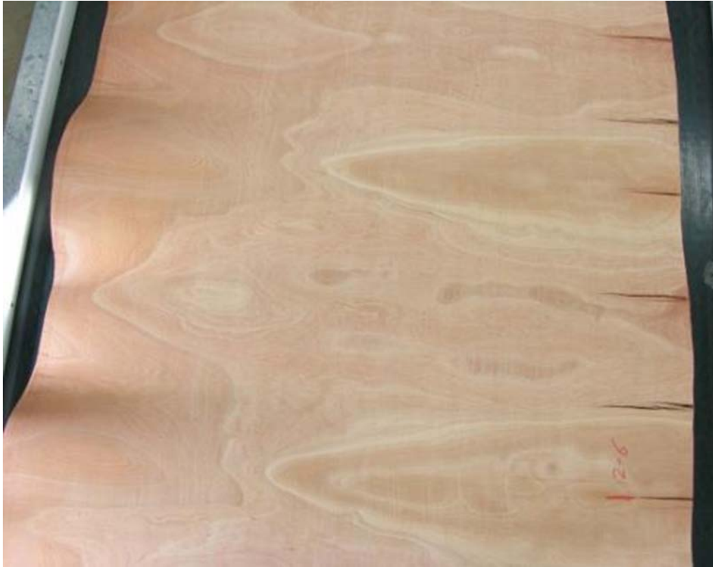
Figure 8.3 Buckling and splitting on opposite edges of the veneer ribbon.
