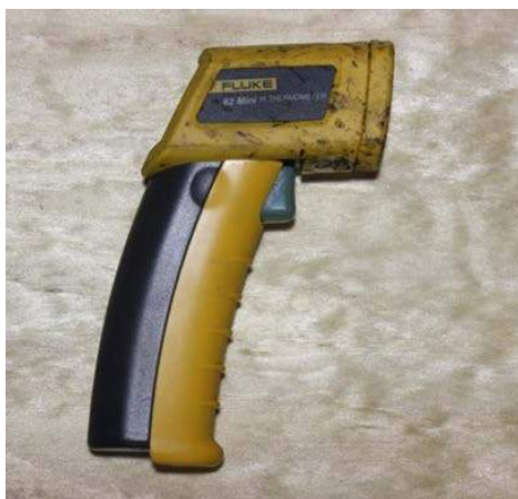
Figure 4.7 An infra-red, non-contact thermometer measures wood temperature safely.
