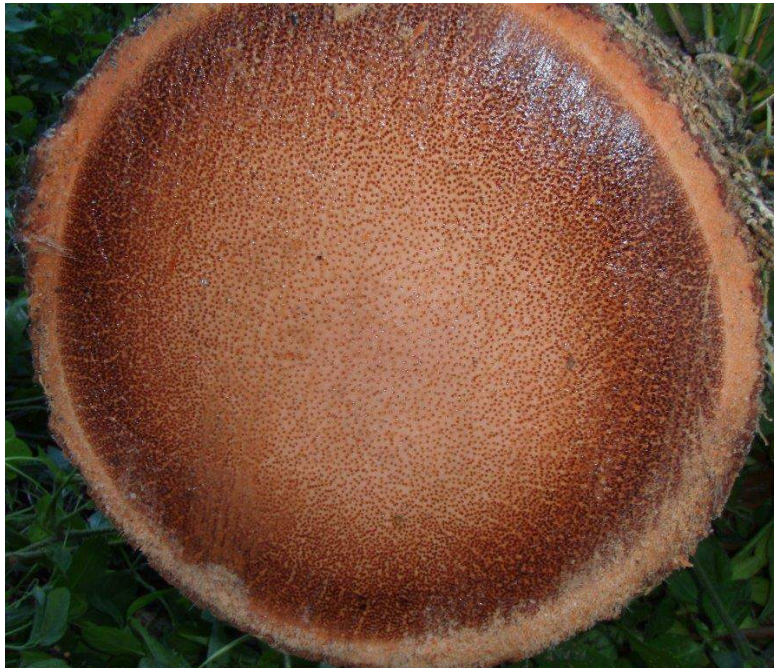
Figure 3.6. Cross-section of a coconut palm stem showing the frequency of vascular bundles increasing radially from the centre to the periphery, corresponding to increasing density.
