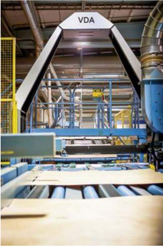
Figure 8.9 Examples of industry in-line moisture measurements of veneer.
