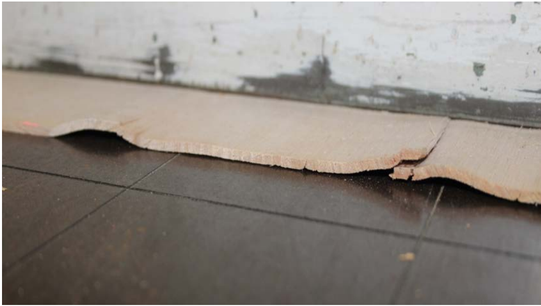
Figure 7.5 Waviness can cause an overlapping when pressed flat.
