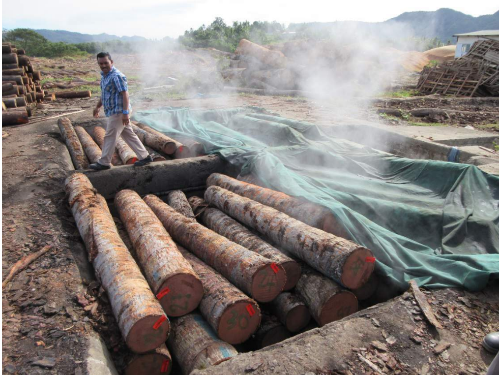
Figure 4.6 Coconut peeler billet pre-conditioning using a steam chamber.
