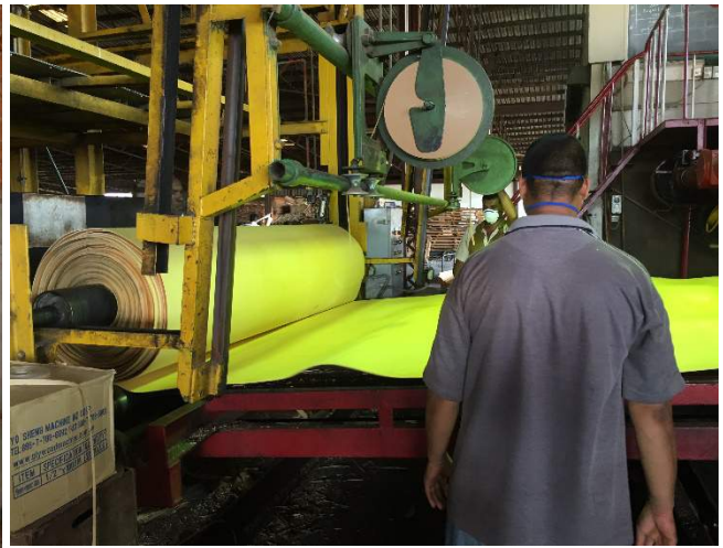
Figure 6.2 Veneer being coiled in preparation for a separate clipping operation.
