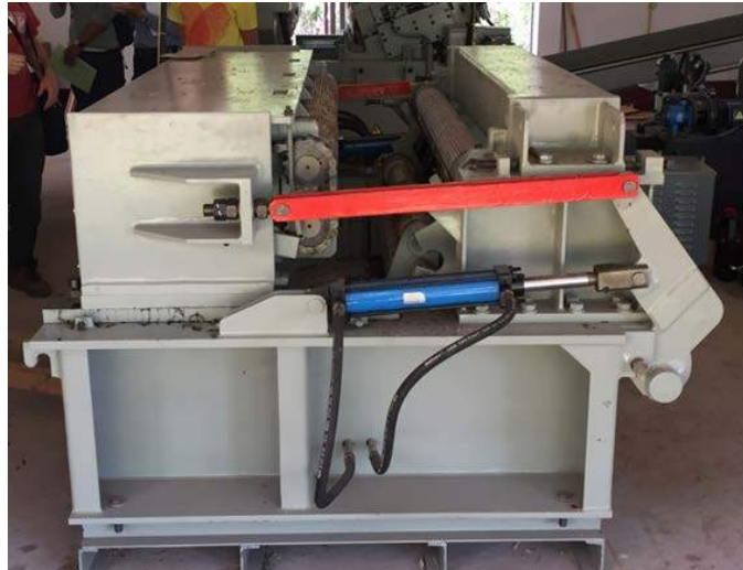
Figure 4.5 Spindleless lathe debarker
