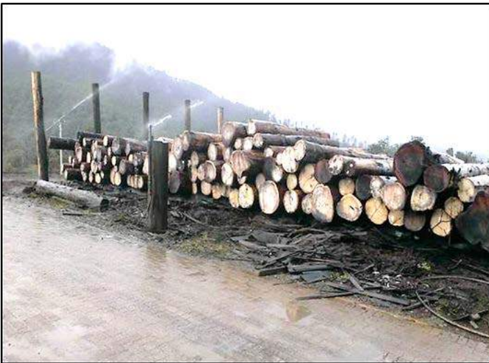
Figure 4.2 Using water sprays in a hardwood log storage yard to prevent excessive, rapid drying and to deter insect and fungal attack.
