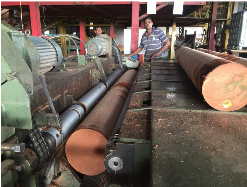
Figure 4.8 Cylindrical coconut logs after round-up, and ready for peeling.
