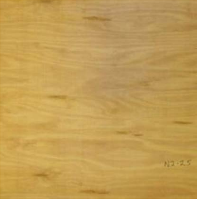
Figure 7.8 Example of the visual quality of B-grade hardwood veneer.
