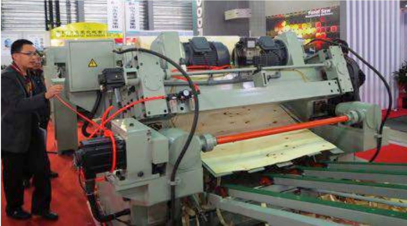
Spindleless lathe peeling on temporary set-up at Shanghai wood Expo
