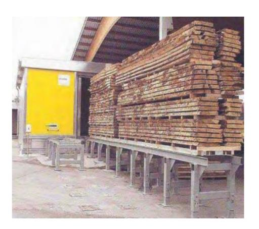
10 m<sup>3</sup> gas-assisted solar kiln was installed at Forestry Department to run research trials (\$100,000 FJD).
