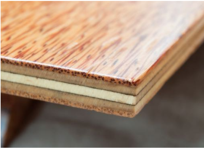
Advanced veneer and other product from coconut wood
