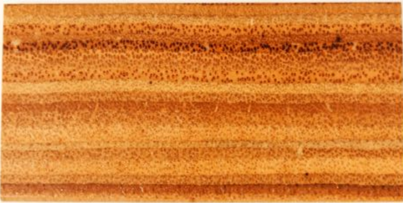
Advanced veneer and other product from coconut wood
