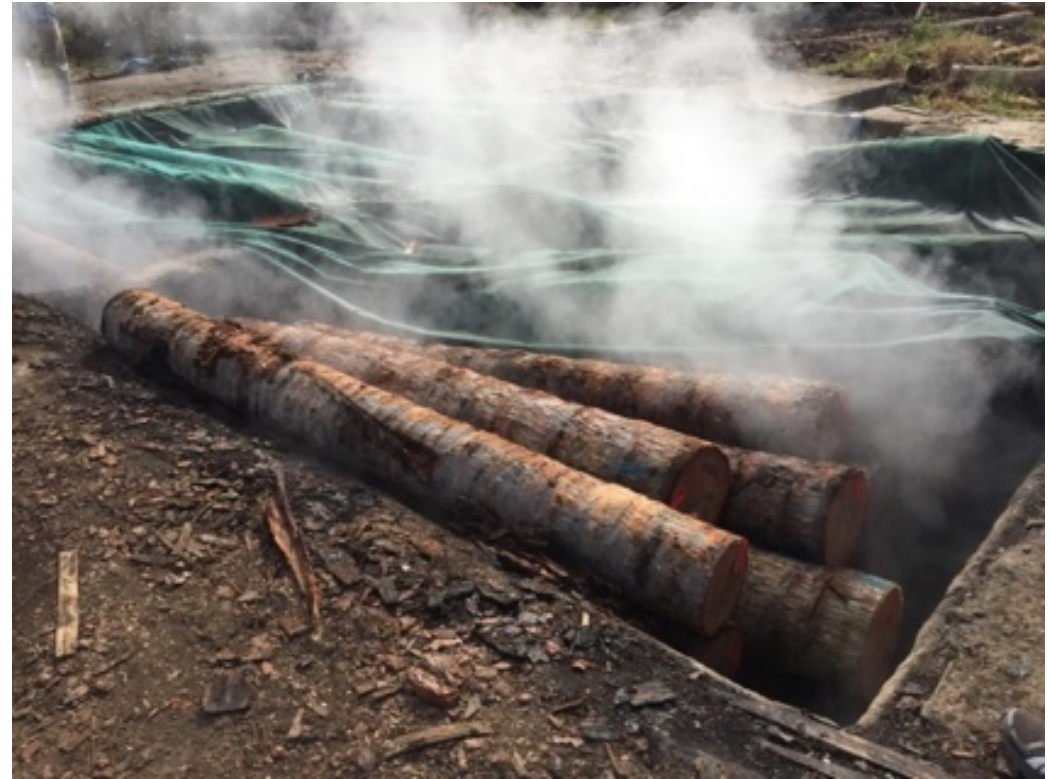
Boiler-driven steam chambers: VTB Labasa
