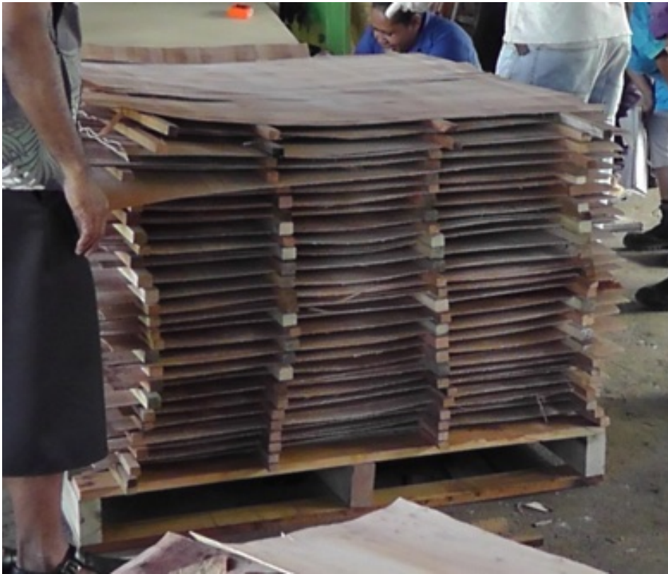
Veneer racked for air drying
