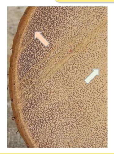
The wood consists of high density vascular bundles in a matrix of spongy, low-density, parenchyma tissue. There is low radial and tangential connection between bundles.
