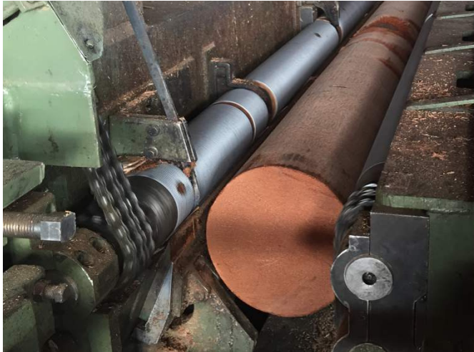
Figure 3. Harvested coconut stems being peeled using a spindle-less lathe
