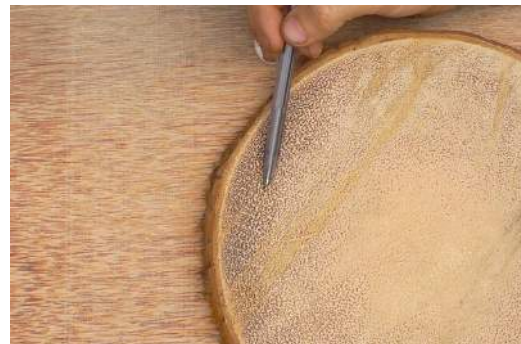
Figure 2: Coconut log disk and veneer illustrating the concentration of vascular bundles on the log's perimeter
