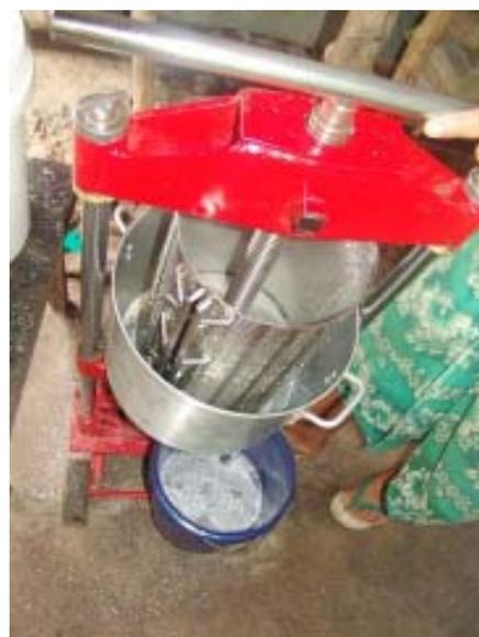
The equipment used for extracting fresh coconut oil, minimal or low heat is used to dry the meat before the oil is extracted by pressing.
